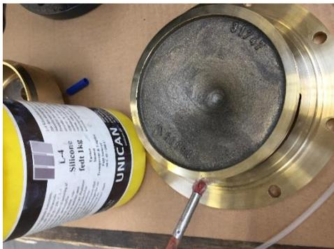
Assemble cone and lower seat
