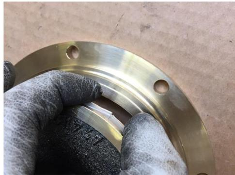
Assembly the O-ring with correct length – USE SILICON
