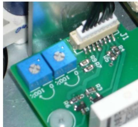
Switch on power supply. Adjust the switch positions with the trimmers R1 (Retract) and R2 (Extend). The relay is switching when the switching position is reached or passed. The switching point can be adjusted from 0 to 100 %. The actuator doesn't need to be re-calibrated.
