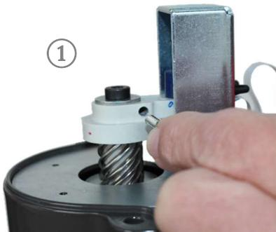
① Screw the ball pin in the drilled hole of the magnet holder by using an open-end wrench (size 5,5 mm).
