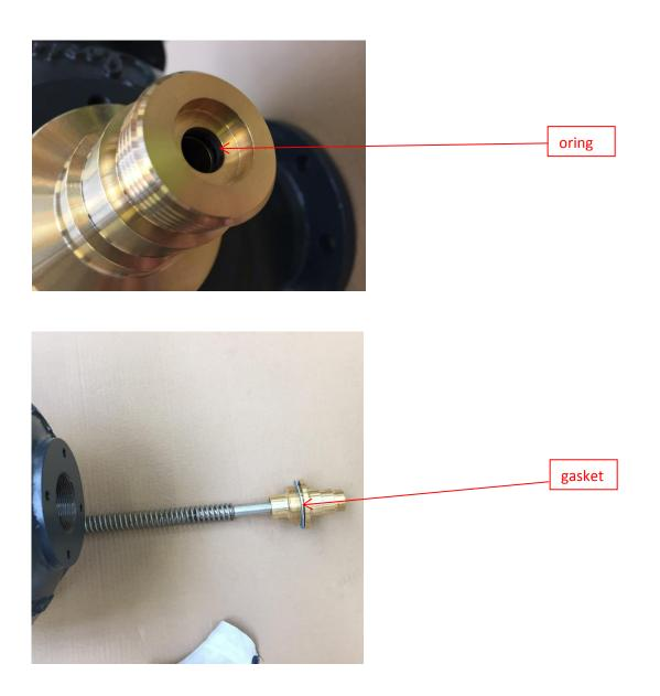
Replace the O-ring tube of lower seat
