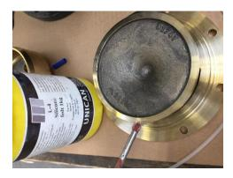
Assemble cone and lower seat
